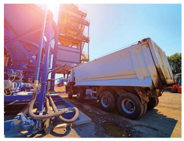
The point of transfer from the mixing plant with material transfer vehicles.
